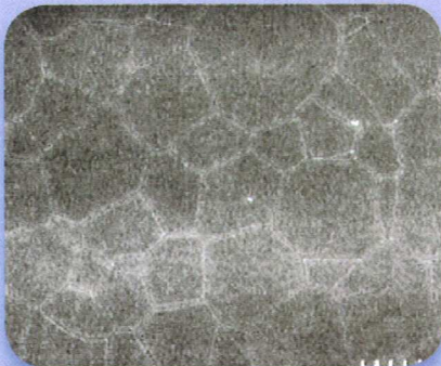
Figure 3 : Polycrystalline structure of highly transparent YAG ceramic after vacuum sintering.
