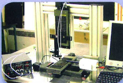
Figure 4 : Powder suspension dispensing system.
