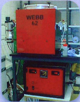
Figure 1 : RED DEVIL Vacuum Furnace.
