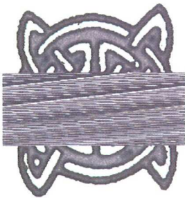
Figure 4 : LTCC goes Celtic: a demonstration of the CO 2 laser precision machining capabilities. Structure is 2mm wide.
